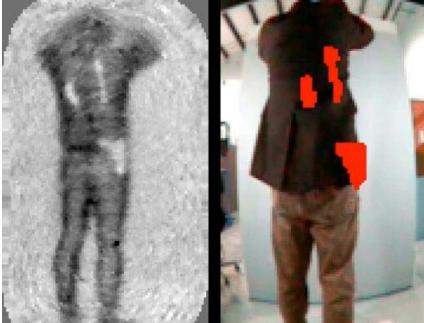
Millivision's scanner marks hidden objects in red on a video image (right); other systems outline a person's body (left). (Millivision Inc.)
